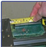
Some lathes have a recessed cross slide, by measuring the gap we may be able to use a slim profile scale to fit within the
