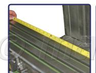
The overall length of table & gap between any table drains. To ensure the scale is easier to fit on the machine. Measure maximum length scale that can be fitted on each axis.
