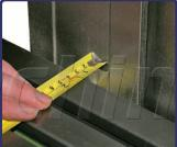
The minimum distance between the rear of the table and column. Depending upon available space it may be necessary to select a slim profile scale or mount on the front of the table.
